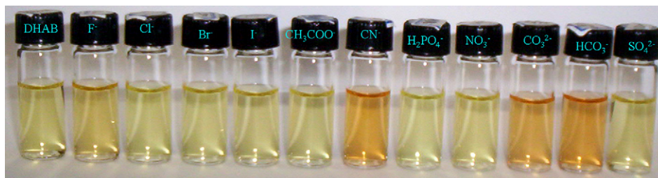
Figure 4. Photographs of DHAB ( 3 \times 10^{-5} M) in a mixture of H 2 O/MeOH (1/1, v/v, 10 mM HEPES at pH 7.5) in the presence of various anions ( 6.0 \times 10^{-4} M). Anions from left to right: blank, F - , Cl - , Br - , I - , CH 3 COO - , CN - , H 2 PO 4 - , NO 3 - , CO 3 2- , HCO 3 - , and SO 4 2- .
